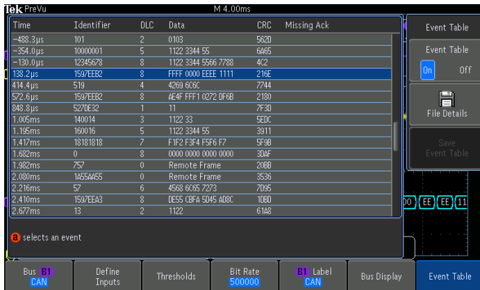
Event table showing decoded identifier, DLC, DATA, and CRC for every CAN packet in a long acquisition.
